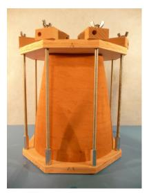
The photo to the left shows the 12" press being used to clamp an 11" tall project.
