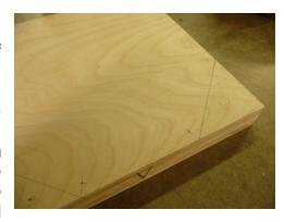
mark the locations to be drilled. Nail the two pieces together with two nails in each corner and one in the middle. Mark one edge with a down arrow. It will become an up arrow then the press is assembled and it is used to align the two pieces. This size works for clamping projects up 11" in diameter and 10  $\frac{1}{2}$ " square.
