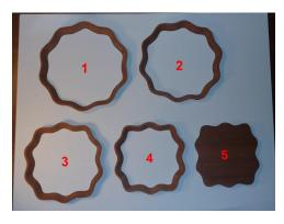
With the angle set start cutting the rings. My choice of blade would be the Olson #9 Precision Ground Tooth (PGT). There are nine cuts to be made that result in four rings and a base.
