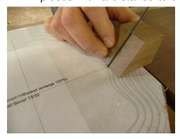
single piece with an angle distance of  $^{7}/_{16}$ ".) If necessary, cut the top off the block to fit under the saw arm. Place the block on your saw and use it to set the angle. With the angle set cut a piece of scrap wood and use it to set the entry hole angle on the wood. Use a  $^{1}/_{16}$ " bit to drill the four holes marked on the pattern.
