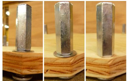
Use 3/8"-16 threaded rod to make posts. Threaded rod comes in length of one, three, or six feet. A three foot piece can be cut to make eight 4 1/2" pieces. This is tall enough to clamp six pieces of 3/4" lumber as is sufficient for most applications. I require being able to clamp thicknesses up to the 6" and also 12". So I used eight pieces of foot long rod for the 12" pieces and cut four rods, cut in half, to make the 6" pieces.
